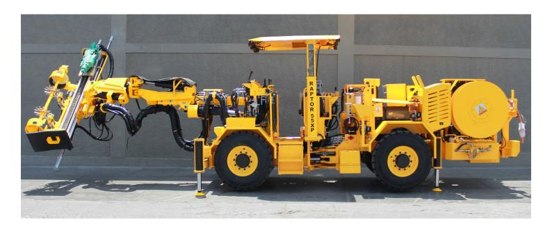
RAPTOR 55 XP is an electro-hydraulic rig for long hole drilling, It has an hydraulic boom, 5APC model, with parallel holding. Use a Montabert Drifter HC 95 with 22 kW and Back -Hammering-rods extractor, the most modern rock drill in the market.
