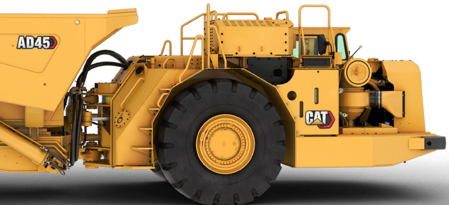
**The new AD45 underground articulated truck is powered by Cat® C18 engine with scalable emission solutions. The truck delivers proven operating efficiency with improvements of serviceability.**
