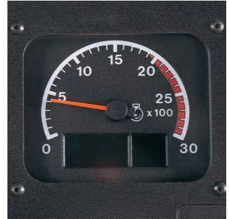
• **Speedometer/Tachometer Module.** Monitors three systems: engine speed, ground speed and gear indicator.
