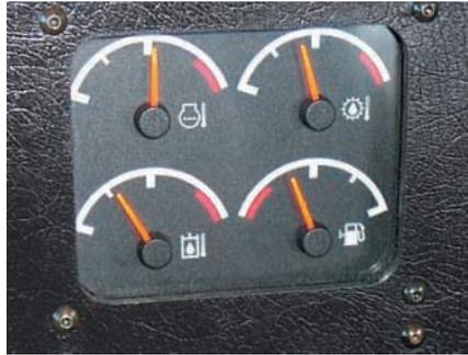
• **Gauge Cluster.** Maintains a constant display of vital machine functions, including: engine coolant temperature, transmission oil temperature, hydraulic oil temperature, and fuel level.
