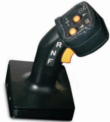
**Ergonomic Layout.** The R1300G II operator station is ergonomically designed for total machine control in a comfortable, productive and safe environment. All controls, levers switches and gauges are positioned to maximize productivity and minimize operator fatigue.
