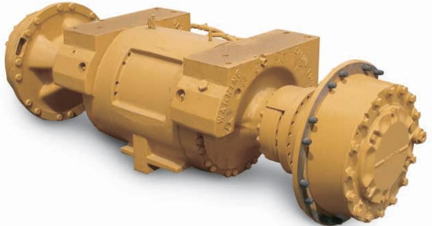
**Final Drives.** Cat final drives work as a system with the planetary power shift transmission to deliver maximum power to the ground. Built to withstand the forces of high torque and impact loads, double reduction final drives provide high torque multiplication to further reduce drive train stress.
