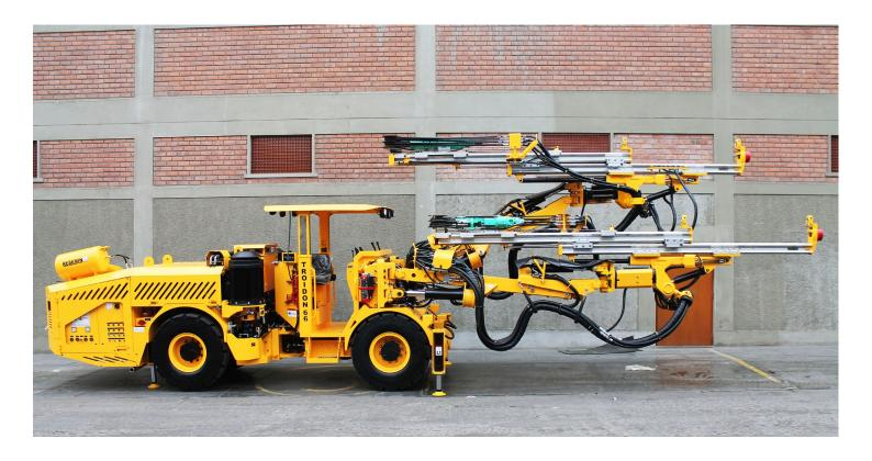
TROIDON 66 XP is an electro-hydraulic jumbo with two booms with automatic parallelism with coverage of 46 m2 drilling.
