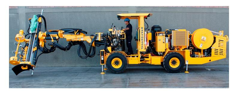
RAPTOR 44 XP is an electro-hydraulic rig for long hole drilling, It has an hydraulic boom, 4AP model, with automatic parallel holding.
