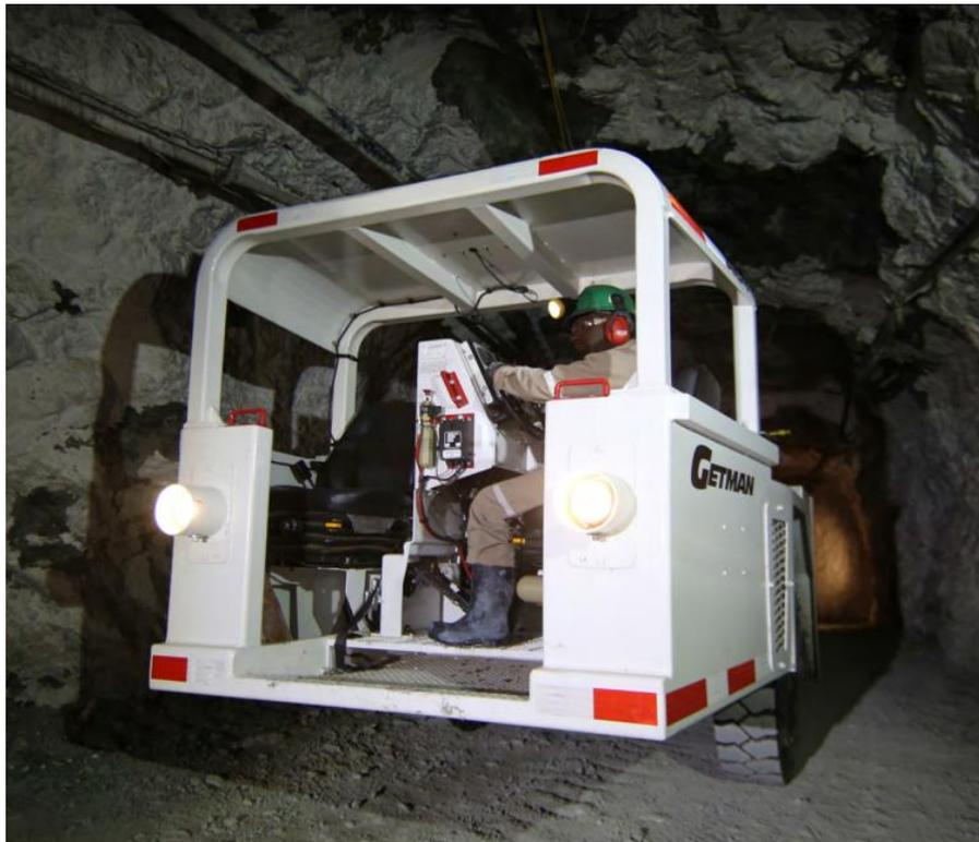
*Getman personnel carriers are designed to support underground logistics by moving crews throughout underground mines safely and efficiently. Built on the reliable A64 Chassis, these carriers protect miner safety through purpose-built design, including individual seat belts for all passengers, a calculated ROPS/FOPS structure over the rear passenger area and a certified ROPS/FOPS structure over the driver compartment.*
