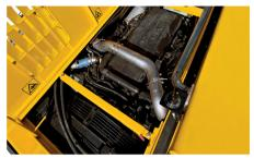
4 final and EU stage 4 approved Cummins QSx15 (for markets with ultra low sulphur diesel and low ash engine oil).
